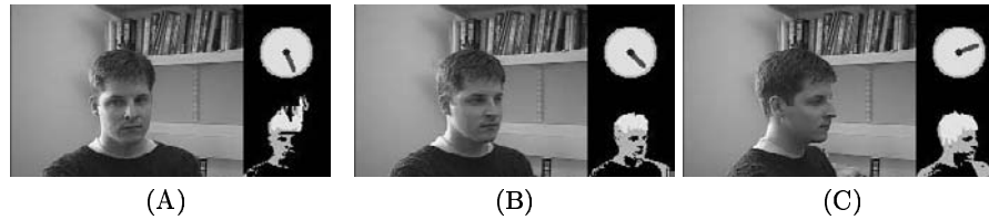
Fig. 6. (A) Pose Estimate for a Misidentified Hair Contour; (B, C) Estimation of a Class 2 Pose Angle Using a Class 1 Projection
