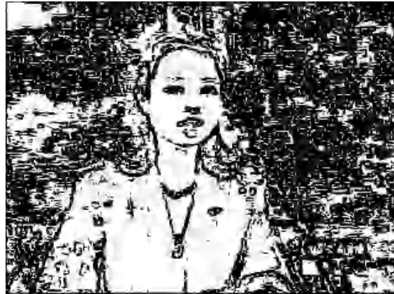
Fig. 5. Binary edge image using an adaptive Sobel operator
