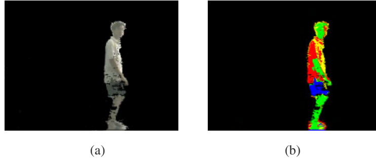
Fig2. Initial segmentation results: (a) The frame after human detection (b) The frame after EM segmentation.
