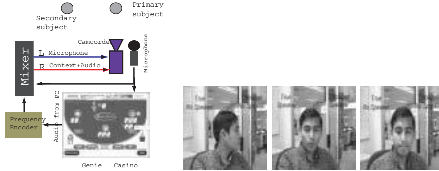
Fig 4. Data collection setup for Genie Casino kiosk and three frames from a test video sequence.
