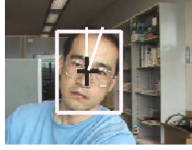
Fig. 2. Moment-based feature of facial region. The position of gravity center, the long-axis angle and the bounding rectangle are shown.
